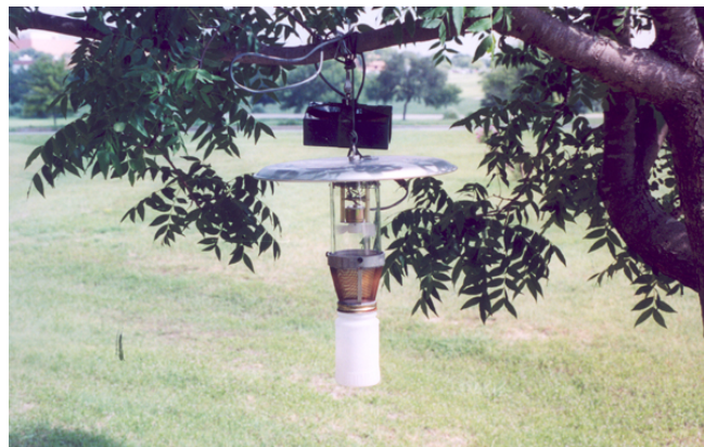
Figure 5. SSAM trap with collection jar shown properly suspended from tree limb.
