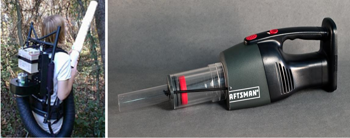
Figure 21. A backpack mechanical aspirator, left (John Hock Co.), and a hand-held mechanical aspirator, right (BioQuip).
