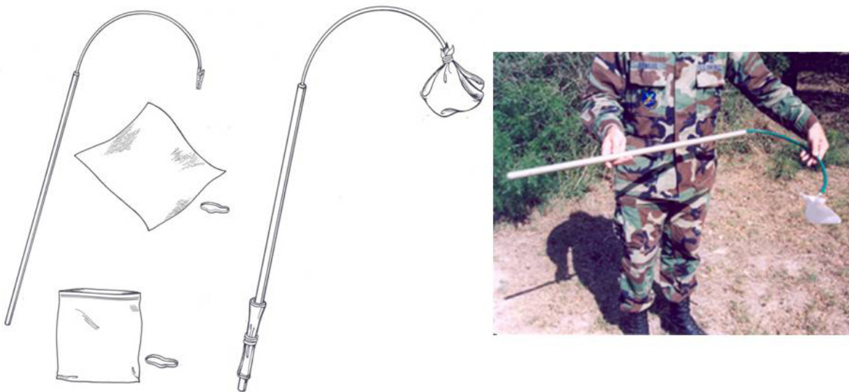
Figure 32. Illustrations and photo of a burrow swab and its component parts.
