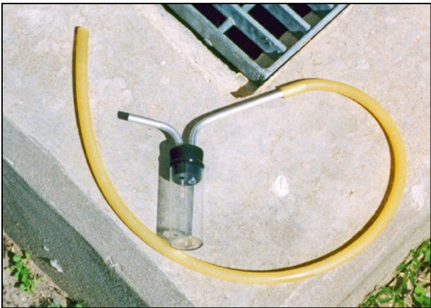
Figure 23. A traditional, mouth-operated aspirator.
