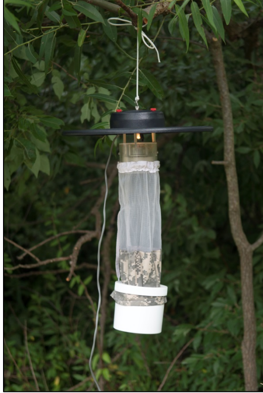
Figure 1. CDC miniature light trap with collecting bag. Photo: SSG Walker, USAPHC..
