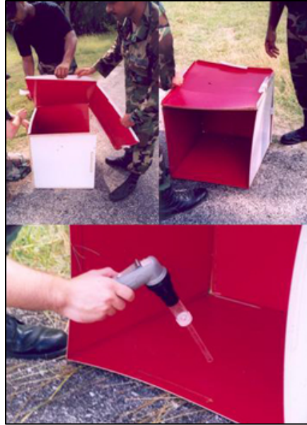
Figure 20. A collapsible red box being assembled and collection of resting mosquitoes with a mechanical aspirator.
