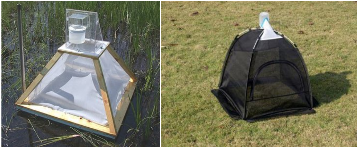
Figure 18. Examples of emergence traps.
